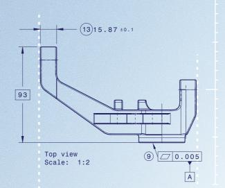
Many manufacturing organizations use 2D drawings to communicate **three-dimensional requirements** to their 3D measurement inspection teams. 2D drawings are also frequently used to produce legal documentation. They consist of a number of 2D views created from a part's 3D model and include the part's dimensional requirements on each view.
